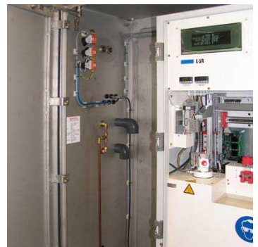
The TOD analyser uses an XY-robot and injection principle
