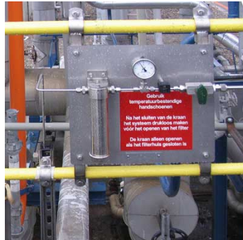
A pre-filter unit to take out big particles and keep sample lines clean
