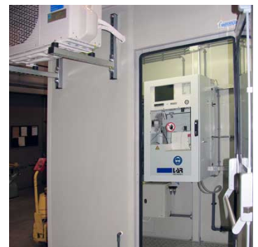
TOC-analyser with loop injection principle; range 0 -1 ppm TC
